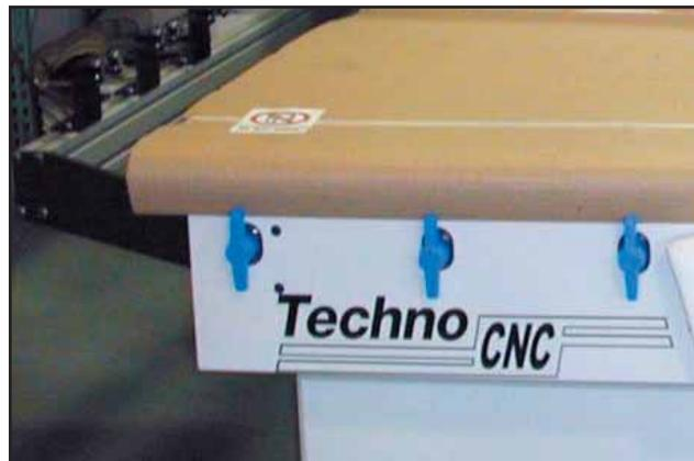
After you have defined your workpiece area and closed off all the vacuum outside of that area, there is another option to greater your vacuum: the vacuum control valves. Each valve controls the flow of vacuum to two rows of extrusions. Turn ON (valve vertical) the valves that pertain to your work area and turn OFF (valve horizontal) the ones outside of that area. This will concentrate all the vacuum “hold-down” capacity to your defined work area.
