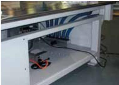
You will need to remove the machine's side panel in order to access and connect the vacuum hose to the manifold fitting (and also if you need to access the servo power box, the vacuum signal connector, etc.)
