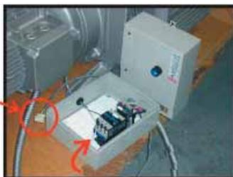
The machine end of the the vacuum signal connector originates behind the front control panel of the RG+ Servo Box 3. This wire needs to be connected to the motor starter's vacuum mating connector. You will need to connect the AC power (220 or 440VAC) to L1, L2, and L3, as specified on the unit here to the Motor Starter connected to its vacuum mating connector.
