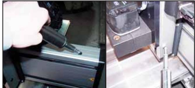
2. Jog the axis to end of travel or until lube point is visible. Using the a grease gun, insert a small amount of grease (see TABLE 2). This lube point greases both the bearing and ball screw simultaneously.
