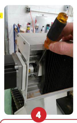
After everything is tight, recheck for backlash. If there is minor or no change, repeat the above instructions. In addition, check all fasteners to make sure they are tight and that there is no other movement in the mechanical assembly.
