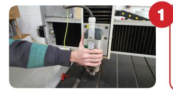
To verify there is mechanical backlash, grab the spindle and try and move it right to left. The stepper motor should be under power so that it prevents the screw from turning during this test. Listen for a small banging noise. If a noise is detected, this means the spanner nut may have backed off the ball screw allowing for the ball screw mechanical assembly to move thus causing backlash.
